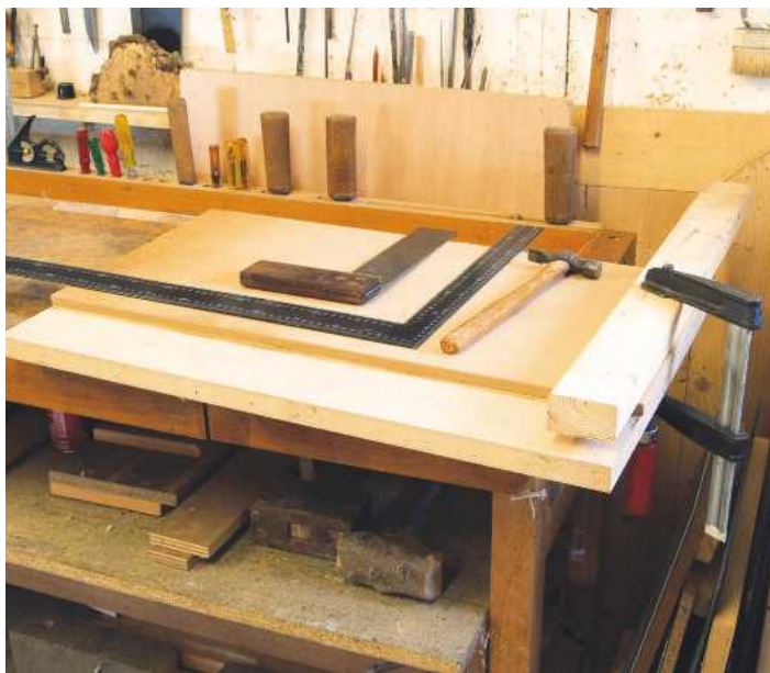
Pic.11 Clamp, check right angle with two squares and tap to make adjustments
